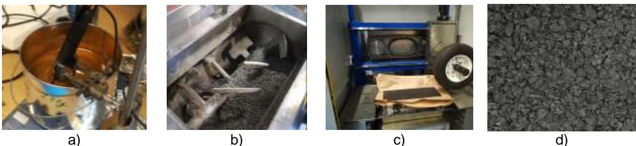
Figure 1: a) Binder Modification with nano-TiO 2 ; b) asphalt mixture production; c) asphalt mixture compaction; d) slab sample of a light-colored pavement.
